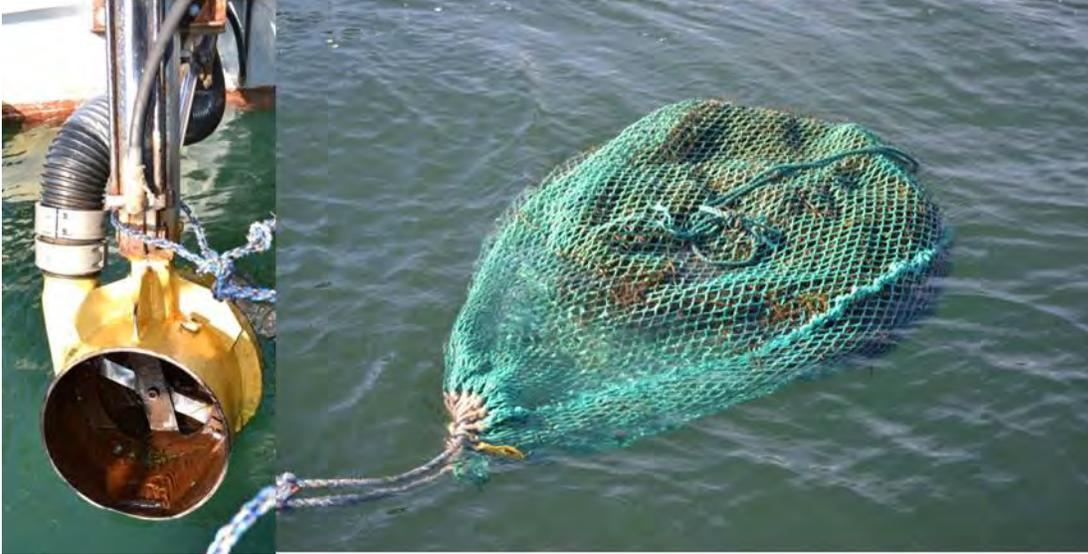
Figure 9. Left. Mechanical harvesting vessel boom cutter. Right. Mesh bag full of mechanically harvested rockweed. Boothbay Harbor, July 2013.
